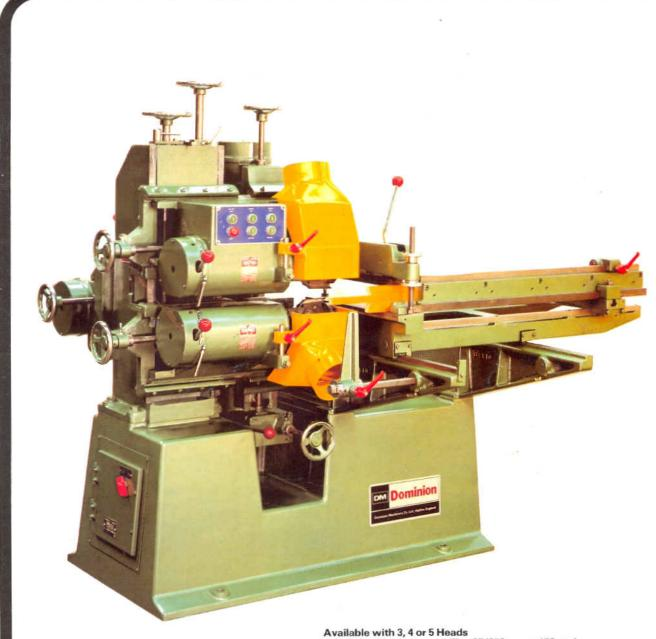
Available with 3, 4 or 5 Heads Admitting Timber up to 14"  $\times$  6" (356mm  $\times$  152mm)
